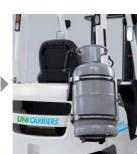
This ergonomically designed swing-down bracket greatly assists in for the lifting and lowering of tanks. The improved design also provides better rearward visibility (available on all LPG-powered models).
