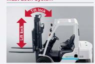
The Mast Lock System, standard on all models, automatically locks all lifting and tilting functions when the operator leaves the seat.
