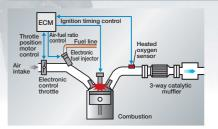
This design includes an automotive-type closed-loop feedback system. Once combustion occurs, a sensor measures oxygen concentration in the exhaust gases before they enter the 3-way catalyst, then sends a signal to the ECM. Based on this signal, the ECM makes the proper air/fuel ratio adjustments, resulting in extremely low emission levels.
